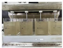
Figure 5: Jar test 4 after 3:30 mins (poly added at 3 mins).
