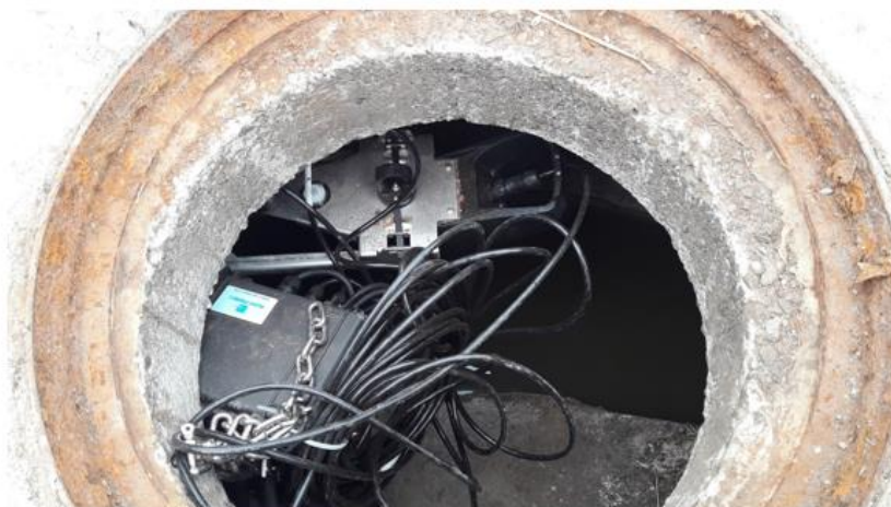
A RavenEye data logger in place capturing flows for use in our waste water modelling
